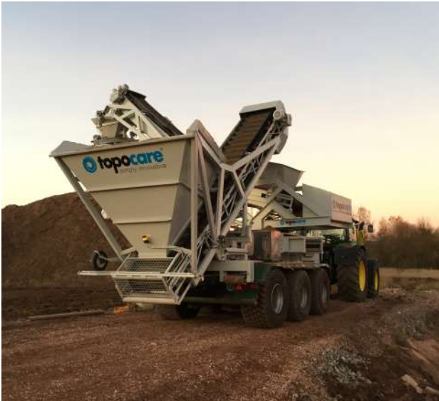
The topomover is a construction machine for producing and laying topotubes.
